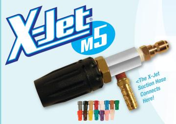
X-JET M5 works just like The Original X-Jet, but the close-range nozzle is replaced by a built-in adjustable nozzle that projects chemicals or other liquids to vertical heights up to 40 ft. at 0° setting or 8 ft. fan pattern at 60° with just a twist. Includes 15 piece proportioner set, shut off ball valve, mushroom strainer and 15 ft. X-Jet Suction Hose with hose barb.
